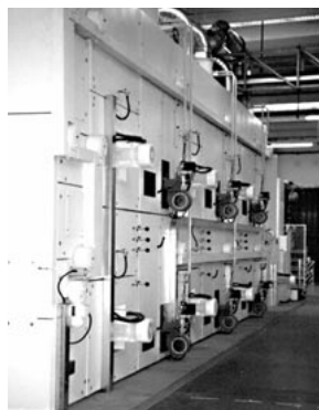
Brückner textile ovens, equipped with compact Eclipse Ratiomatic Burners, Model 50 RM - Version 2.00, are setting a new world standard for environmental excellence.
