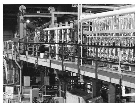
Inland Steel's computer-controlled process includes an annealing oven equipped with 193 Eclipse Auto-Recupe burners, each having a diameter of 7.5 inches and an effective length of 84 inches. Since the furnace upgrade, Inland has experienced improved energy efficiency and compliant emissions.
