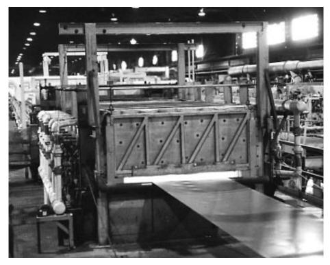
Inland's continuous heat treating line processes the steel within the chambers of this 270-foot-long furnace. Depending on the alloy, temperatures range from 1500° to 1800° F. After annealing, a chilled atmosphere of nitrogen and hydrogen cools the steel to about 400° F.
