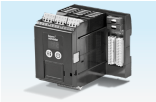
Once the plug-in power module has been removed, the parameter chip card and fuses are accessible.
