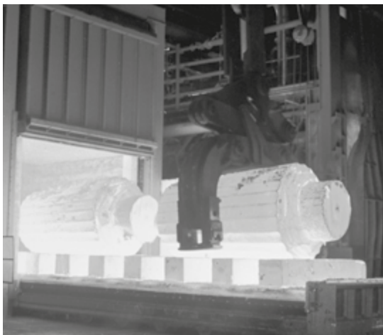
Steel forging furnace
