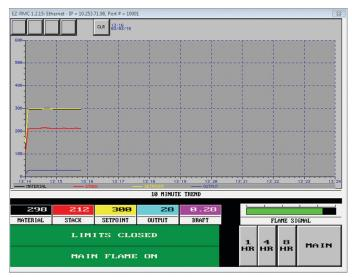
Trend of set point, material and stack temperatures and burner output from BCS-7000
