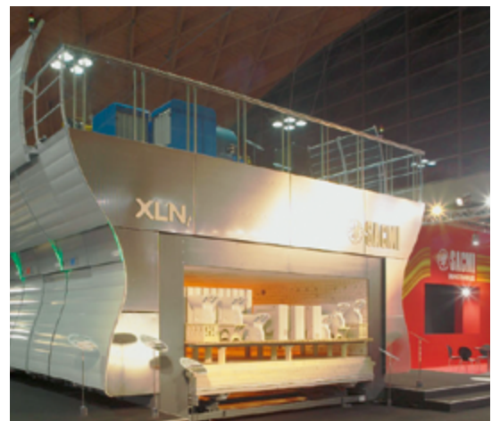
Roller hearth furnace
