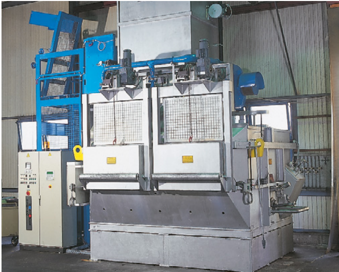
Aluminium industry: shaft melting furnace
