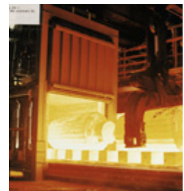
Butterfly valve BVHM on forging furnace to re- duce the oxygen level
